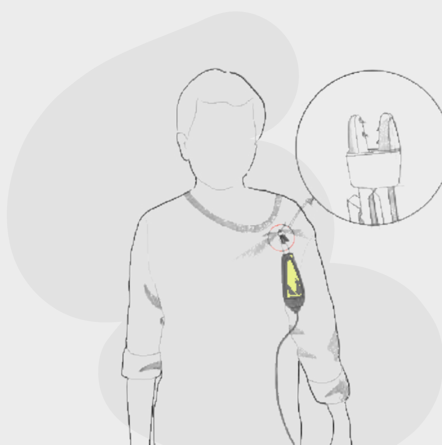
Sharp teeth on clamp tears the clothes
